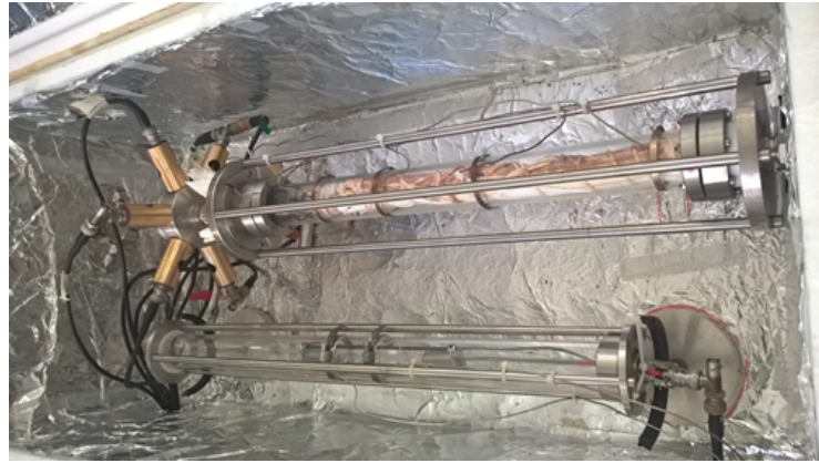
Figure 7. Photo of the air flow calorimeter with both reactor ( top ) and calibration lamp ( bottom ).
